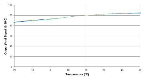
7H Hydrogen sulphide CiTiceL - Baseline vs Temperature
